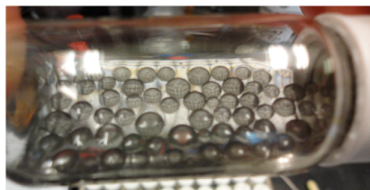
Figure 1. Pickering emulsion of water in heptane stabilized by pristine, natural flake graphene. The ratio of heptane to water is 19:1.
